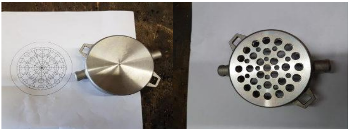
Filter for prevent bolts and nuts entering into the flow gauge
