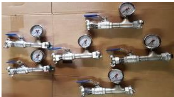
Steam pipe Testers with drag needle pressure gauge
